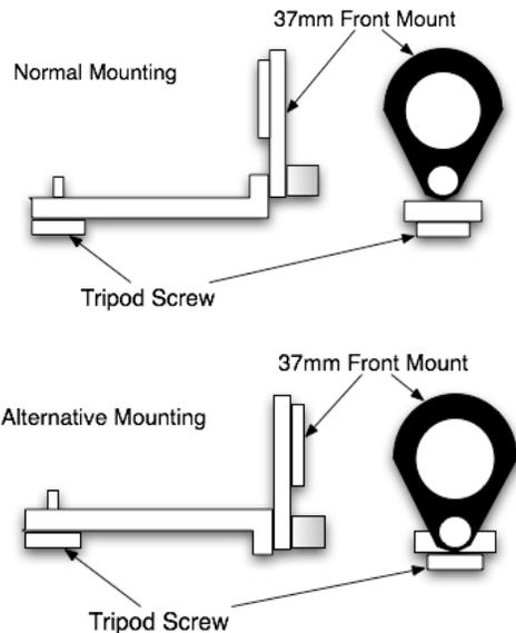
The Xtend-a-Lens OMNI comes partially disassembled and can be put together as above. Note that there are several options possible with the flexible design of the unit. **THE BOTTOM RAIL CAN BE FLIPPED UPSIDE DOWN TO EITHER GAIN ADDITIONAL HEIGHT OR LOWER THE HEIGHT OF THE FRONT MOUNT DEPENDING ON THE LOCATION OF THE CAMERA LENS ON THE CAMERA.**
